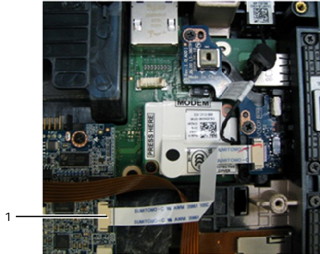
1 Wi-Fi Sniffer cable connection to motherboard
